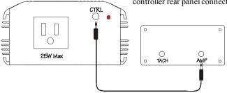
Connect the output of the wall adapter to the amplifier by plugging the 2.1mm plug into the connector on the back of the amplifier marked "24VDC". Connect the wall adapter's AC plug to your house's mains power wall socket. Connect the turntable motor's AC plug to the amplifier output connector marked "25W Max".
